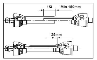
shafts and safety covers. Carefully remove all burrs then clean and re-lubricate before reassembling.
