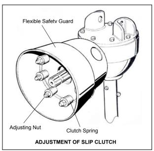
If the post hole digger has not been used for some time and the clutch cannot be made to slip, it may be seized due to sticking plates. In this case, fully slacken each of the clutch bolts and run the digger for about 30 seconds with the auger in the ground to free the clutch plates and clean the surfaces. Then re-tighten the spring bolts evenly to achieve the required slip setting. This can be done by compressing the springs fully and then backing off two turns.
