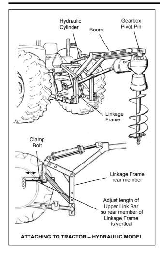
Install the hydraulic cylinder between the lugs on the linkage frame and boom using the pins supplied. Connect the hoses to the tractor, see below for further details.
