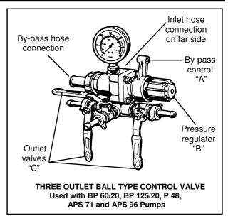
Moving the lever its full travel anti-clockwise directs pressurised fluid to the boom, or any other spray device connected to the system, and only the overflow from the pressure control is recirculated to maintain agitation within the tank.
